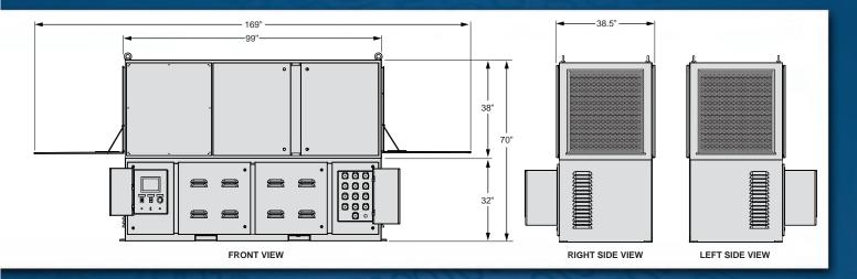
The load bank resistor elements are forced-air cooled with a heavy-duty, three-phase, TEFC electric blower motor with a high-performance direct-drive fan blade. The blower motor can be powered from the main input load bus (test source) or optionally from an external three-phase supply source. Motor starter circuit is fuse protected and includes an overload relay.
